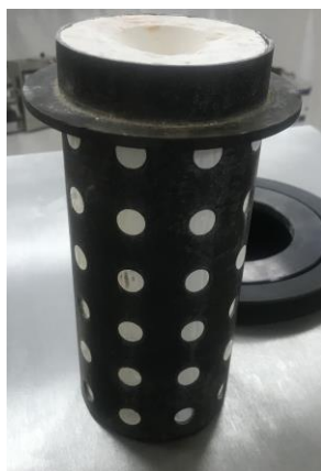
Figure 3. Plaster in the cylinder with holes after hardening and tape removed.
